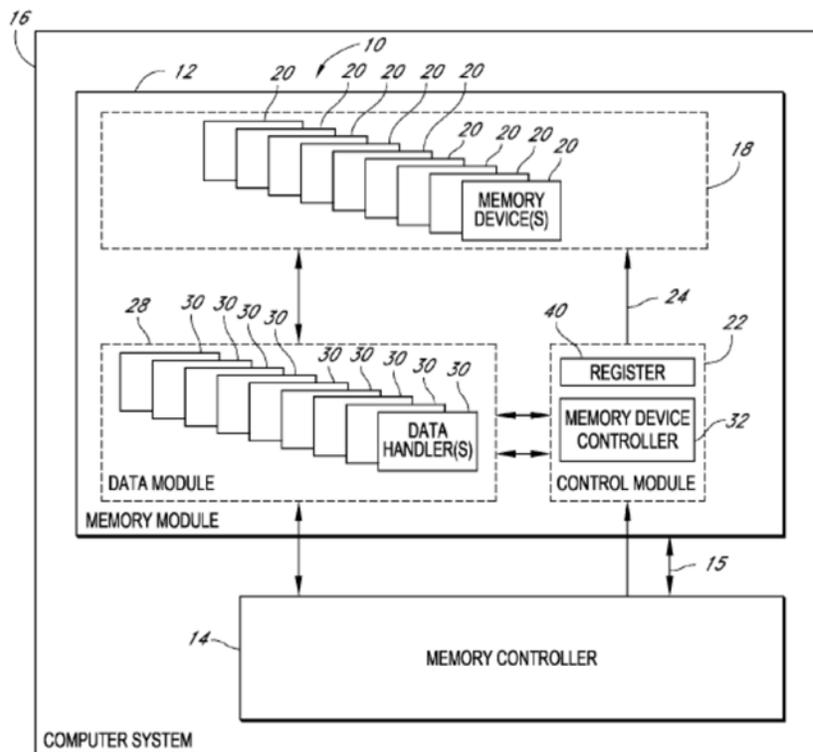
As illustrated in Figure 1, above, “memory module 10 includes a printed circuit board 12 configured to be operatively coupled to a memory controller 14 of a computer system 16.” *Id.* at 5:6–8. Memory module 10
