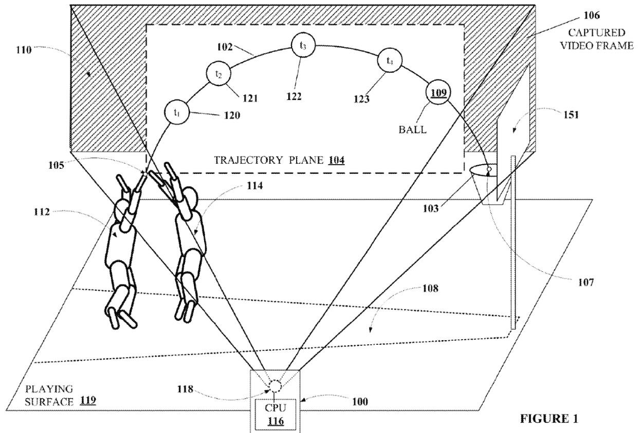
Figure 1 depicts a trajectory capture and feedback scenario employing a trajectory detection and feedback system using a machine vision system with a single camera to detect basketball trajectories. *Id.*, col. 8, ll. 17–19, 58–60. The specification explains that sensor systems other than machine vision systems may be used to generate trajectory parameters. *Id.*, col. 19, ll. 15–
