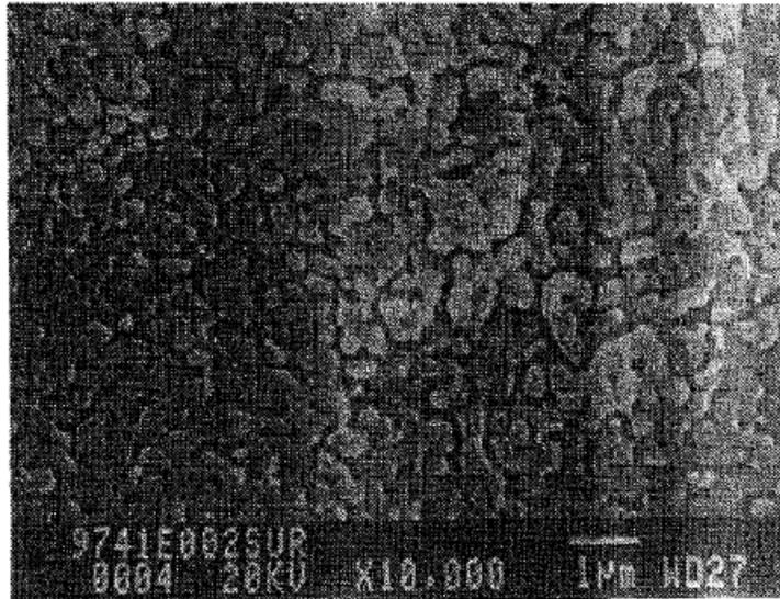
Fig. 5 shows interconnected particles exhibiting porosity.
