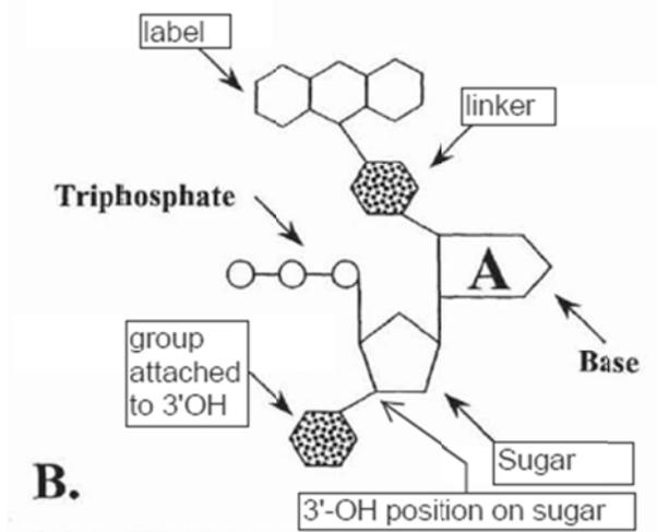
Figure 1B of Stemple shows a generic nucleotide's main parts, including a detectable label ("label"), a linker, and a chemical group attached to the 3'-OH position.
