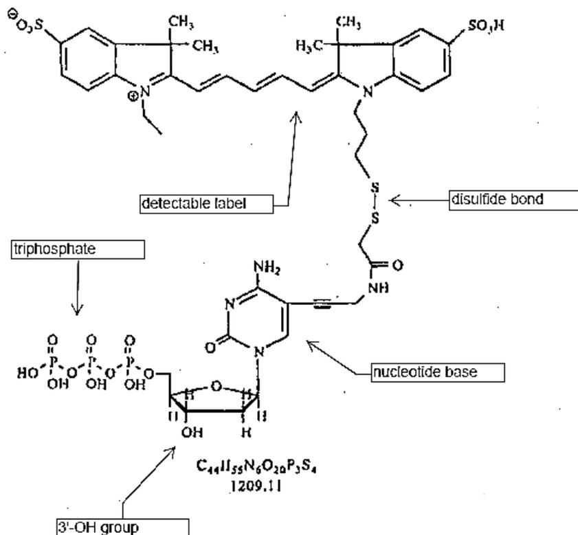
Figure 5 of Church is annotated to identify the structures of the nucleotide, including a detectable label, a triphosphate, and a disulfide bond. Ex. 1019, 17:10–11 (“Figure 5 is a schematic drawing of a disulfide-bonded cleavable nucleotide fluorophore complex.”). The nucleotide, however, lacks the claimed protecting group on the 3'-OH.
