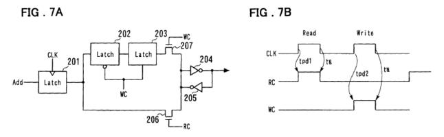
Figure 7A of Takahashi depicts a circuit for introducing delays in an address register. Ex. 1003, 6:46–48, 17:9–14. Figure 7B depicts a timing diagram for illustrating the timing of the circuit in Figure 7A. *Id.* at 6:47–48.
