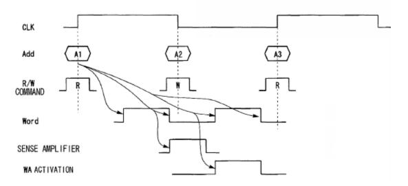
Figure 15 of Takahashi depicts a timing diagram for an alternative embodiment of Takahashi. Ex. 1003, 7:1–2. Takahashi explains that "the read command RE and addresses A1 and A3 are sampled with the rising edge of the clock signal CLK, while the write command W and the address A2 are sampled with the falling edge." *Id.* at 21:10–13.
