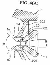
Figure 4A depicts a sectional view of the front end of the paint nozzle tip with an air groove (1a) that starts at a point (102) inside the inlet end (201) of an annular slit (4). *Id.* at 6:40-54.
